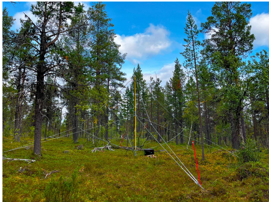
Angeli VLF receiver installed in August 2024 in Inari, Northern Finland.
